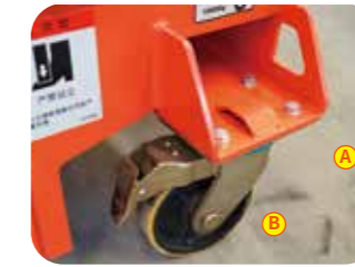
A:Standard forklift pocket
