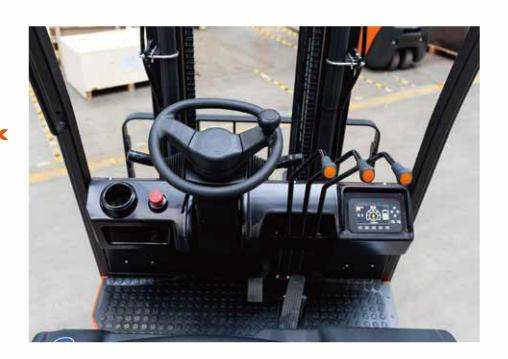
The trucks are equipped with Curtis controllers, **CAN-bus** technology makes the diagnostic and troubleshooting easier.
