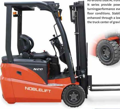
All-around Dual AC front wheel drive motors for the N series provide powerful travel and excellent turningperformance even in the most undesirable floor conditions. Stability of the truck is further enhanced through a low mounted battery keeping the truck center of gravity lower to the ground.
