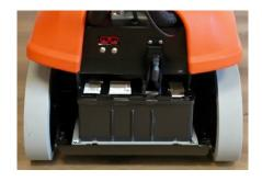
Low energy consumption control system. A full charge can run the machine for 1.5-2 hours on a standard 24V/32AH leadacid battery.
